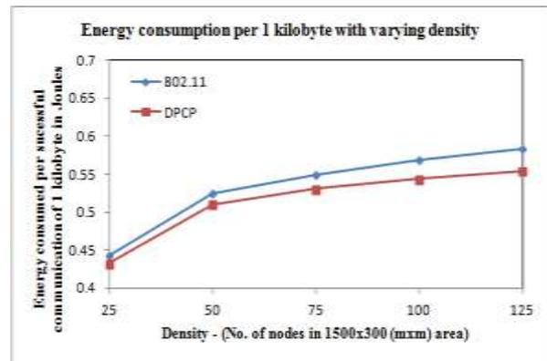
**Figure 4: Average energy consumption (in Joule) per communication of 1kilobyte of data vs density**
