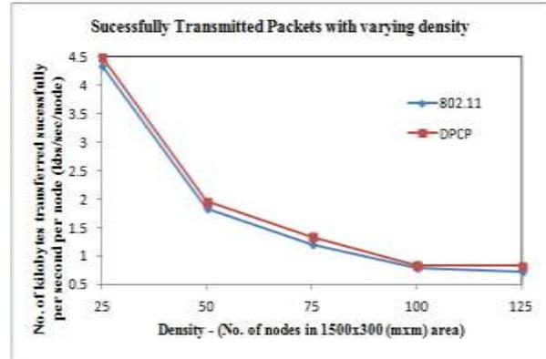
**Figure 3: Successfully 1 kilobyte of data transmitted vs density**
