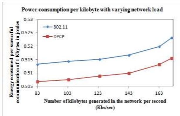
**Figure 2: Average energy consumption (in Joule) per communication of 1kilobyte of data vs traffic generated rate**
