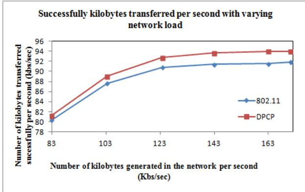
**Figure 1: Successfully data transmitted vs traffic generated rate**
